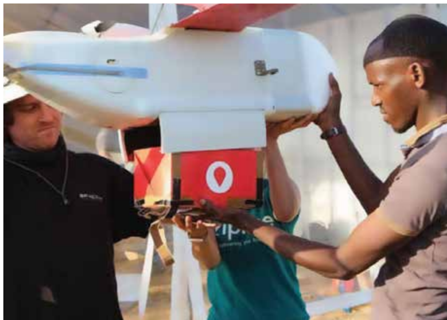
Source: http://www.nation.co.ke/news/africa/Rwanda-begins-to-deliver-medical-supplies-using-drones/1066-3416798-iggtlc/index.html A technician (right) for American robotics company Zipline installs a small cardboard box with a paper parachute in a drone prior to its launch in Muhanga, Rwanda, on October 12, 2016. Rwanda launched drone operations to deliver medical supplies to hospitals in remote areas. PHOTO | AFP
